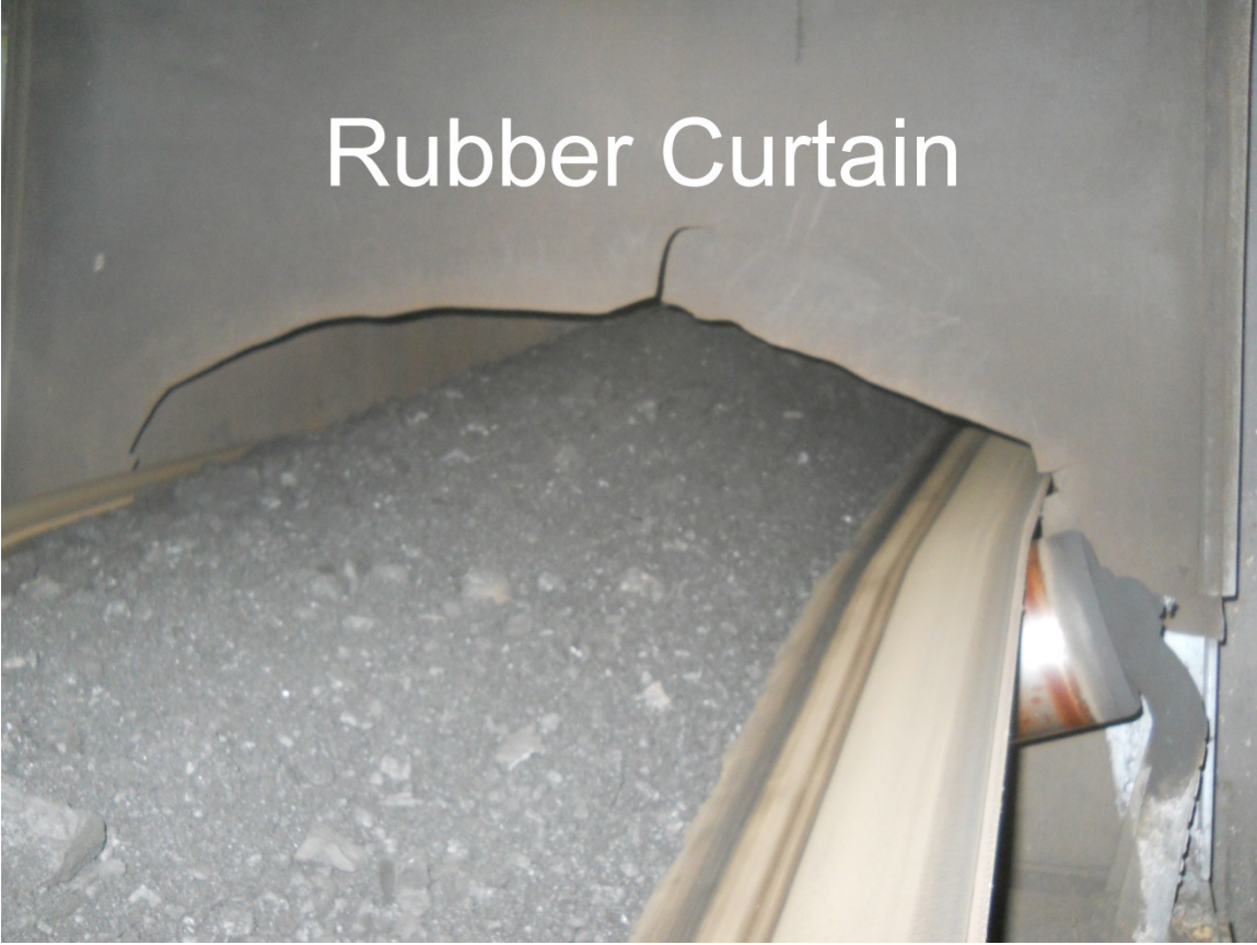
Figure 5.4 Entry and Exit Curtains
