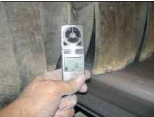
Figure 7.3 Air measurements can be performed with a relatively inexpensive handheld anemometer and a ruler.
